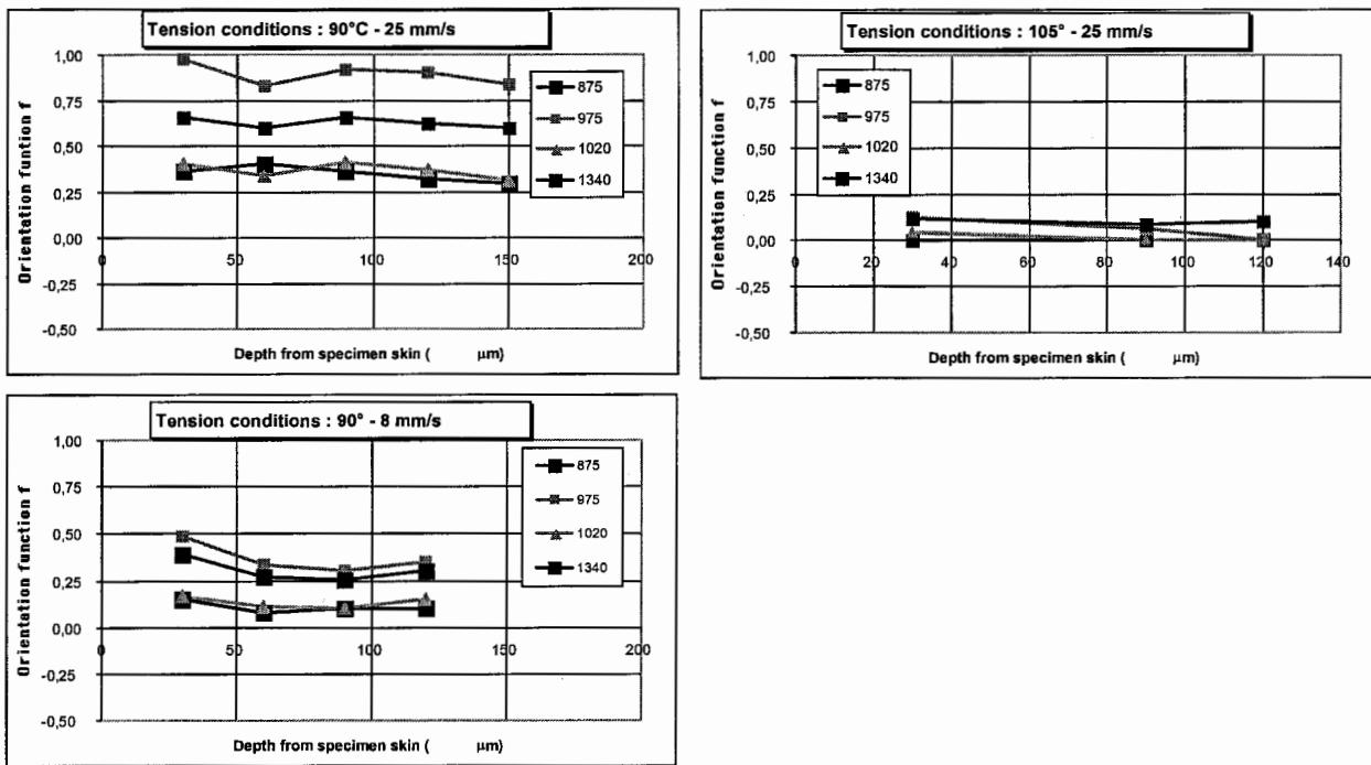
Figure 18: Influence of uniaxial testing conditions on macromolecular orientation. On top plots one can see that from  $90^\circ$  to  $105^\circ$  the final orientation decreases nearly to 0. On left plots one can see a similar influence due to decreasing of tension speed.
