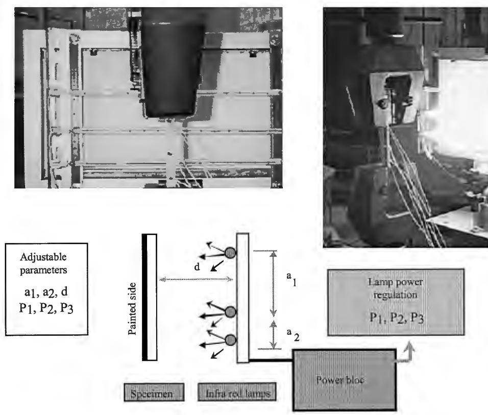
Figure 1: Infra red heating apparatus
