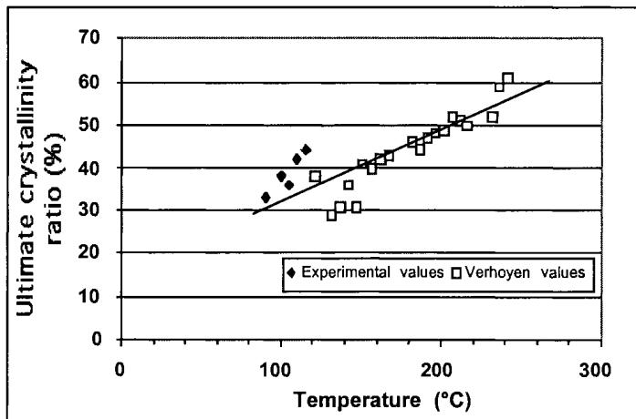
Figure 13: Ultimate crystallinity ratio dependence on temperature
