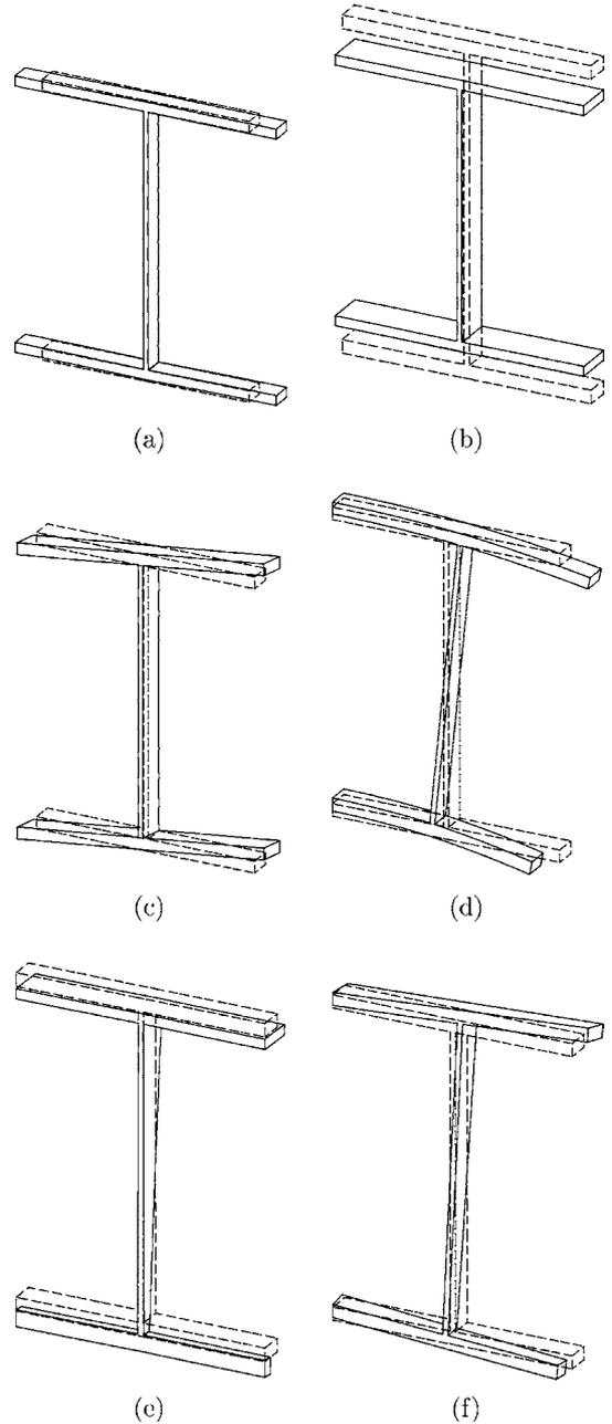
Fig. 5. Deformed shapes obtained from solving the basic cell problems for the panel with straight stiffeners: initial configuration shown in broken line, deformed shape in solid line. (a)  $\chi^{E_{11}}$ , (b)  $\chi^{E_{22}}$ , (c)  $\chi^{E_{12}}$ , (d)  $\chi^{K_{11}}$ , (e)  $\chi^{K_{22}}$  and (f)  $\chi^{K_{12}}$ .
