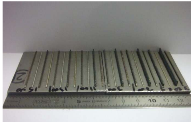
Fig. 1. Image showing multilayer's depositions on a low carbon steel substrate.
