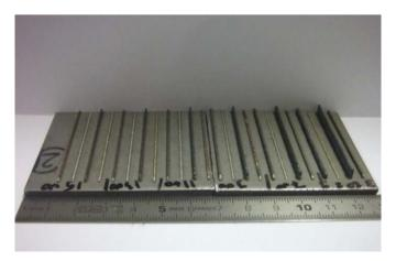
Fig. 1. Image showing multilayer's depositions on a low carbon steel substrate.
