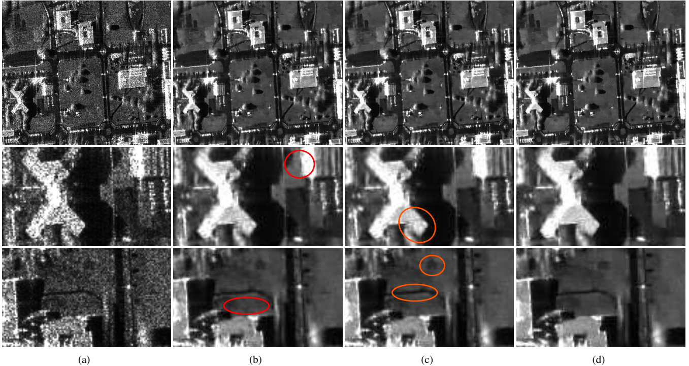
Fig. 3. (a) 2-look SAR image of Toulouse (France) ©ONERA ©CNES (the two images at bottom are zooms of the top one). (b) Result of EPLL applied after log-transform and with a post debiasing step following [17]. (c-d) Result of our approach with a Fisher-Tippet based data fidelity term on the log-transformed data respectively without and with invariance.
