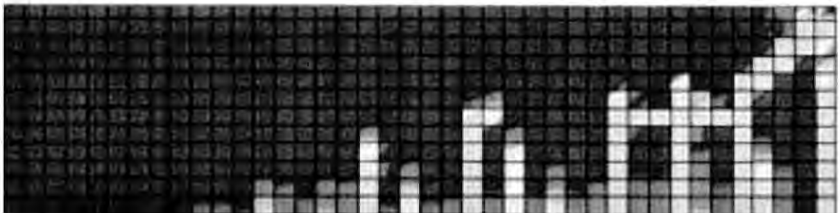
Figure 11. Distribution of damage in a longitudinal cross section. . The load is applied at the top-right corner (axis of symmetry) and vertical displacements are fixed at the bottom left corner
