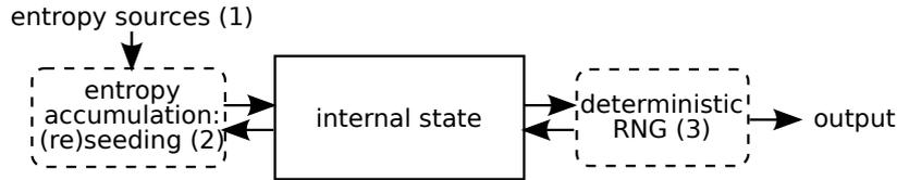
Figure 1: Model of PRNG with entropy inputs.
