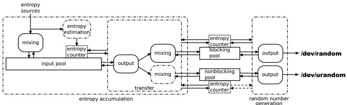
Figure 2: General structure of the Linux PRNG.
