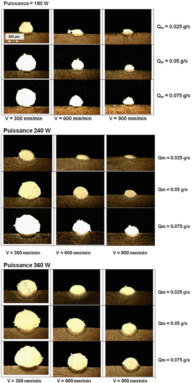
Fig. 7. All single tracks' cross-section. For each laser power the velocity ( $V$ ) increases from the left to the right and the feed rate ( $Q_m$ ) increases from the top to the bottom.
