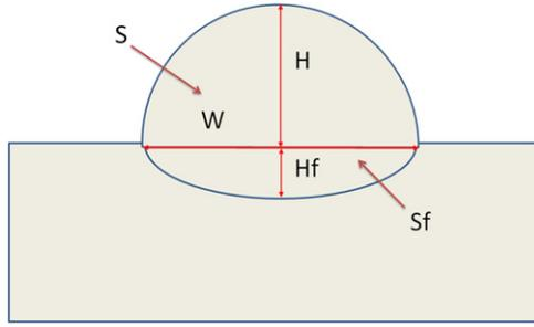
Fig. 6. Cross section measures for each single track.
