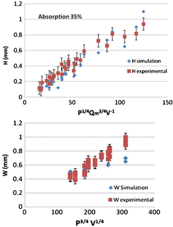
Fig. 17. Confrontation of the experimental height and width with the simulated results in the case of a Gaussian distribution.
