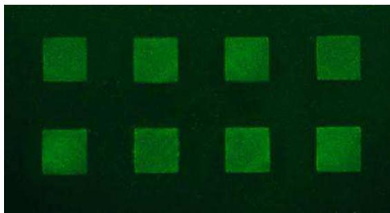
Fig. 3. Fluorescence microscopy picture observed at  $\lambda_{exc} = 550$  nm and  $\lambda_{em} = 570$  nm of diamond patterned by oxidation and functionalized with OBP immobilization after the immersion in a fluorescein solution.
