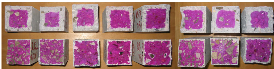
Fig. 13. 1-year natural carbonation fronts of B1, B2, B3, B4, B5, B6, B7, B8 concrete samples. First row: 50% curing conditions. Second row: 24 h - Water curing conditions.
