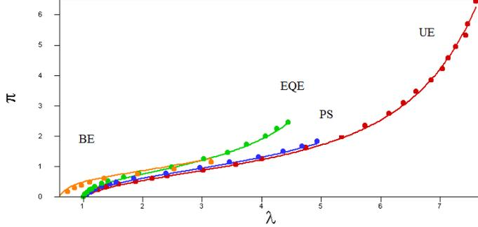
Figure 4. Experimental data ( $\bullet$ ) and GD model identification for biaxial extension (BE), equibiaxial extension (EQE), pure shear (PS), uniaxial tensile extension (UE). Incompressible GD model response.
