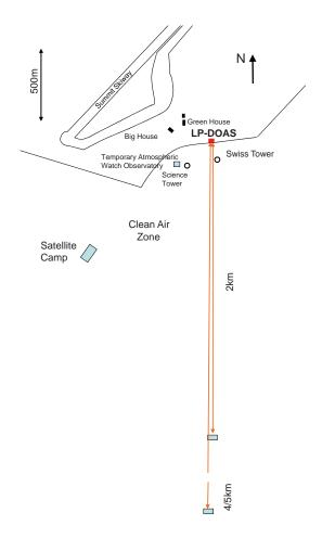
**Fig. 1.** Overview of the LP-DOAS setup during GSHOx.
