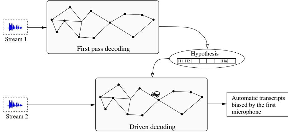
Fig. 4. Driven Decoding Algorithm used with two streams: The first stream drives the second stream
