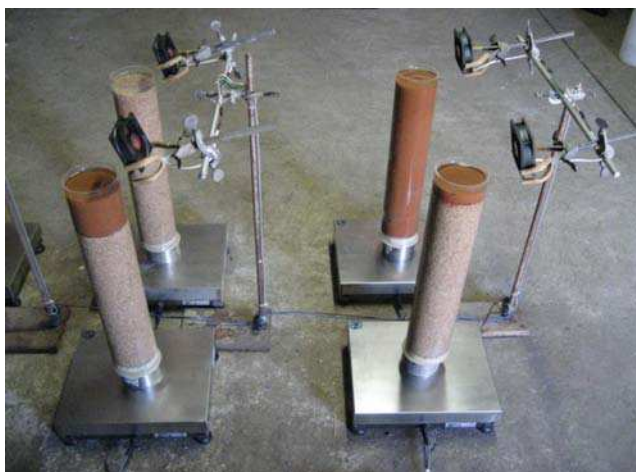
Figure 2. Experimental setup for the homogeneous and the two-layer columns (the brown soil in the sandy loam, and the gray one is the coarse sand). The fans at the top of each column are shown.
