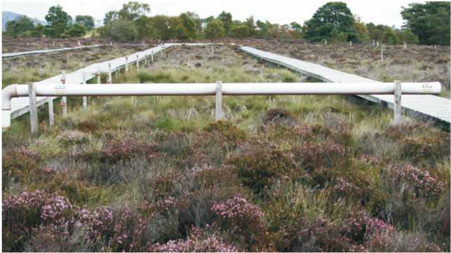
Figure 5.22: Photograph (taken on 27/08/09) looking downwind of the 60m ammonia free air release transect at Whim Bog, a lowland raised bog in the Scottish Borders. The photo shows the undamaged vegetation upwind of the 6m release pipe and the change in vegetation with the loss of Calluna vulgaris , Sphagnum spp. and Cladonia portentosa up to 24m downwind of the \text{NH}_3 release point, which is now dominated by Eriophorum vaginatum . © Ian Leith
