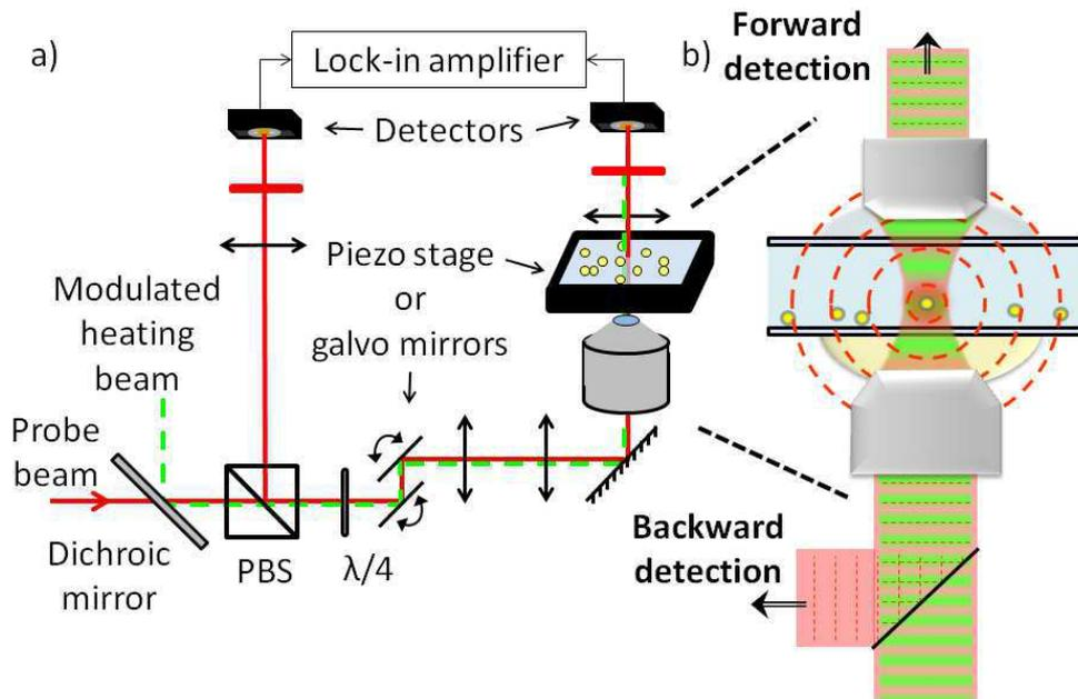
**Figure 1: a) Typical photothermal setup (PBS: polarizing beam splitter,  $\lambda/4$ : quarter wave plate) with b) backward and forward configurations.**
