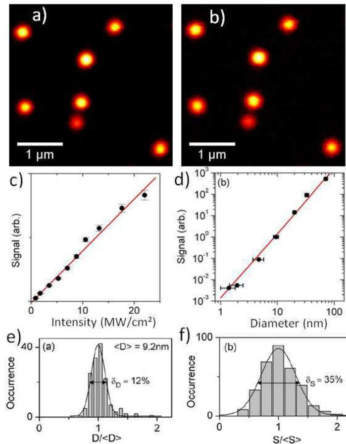
**Figure 2: PhI images and dependences. a) and b) Images of 10 nm gold nanoparticles deposit on a glass slide, in the forward (SNR = 322) (a) and backward (SNR = 62) (b) configurations. Photothermal signal dependence with c) heating power, measured from a single 10 nm nanoparticle and d) particle size. e) Diameter D (TEM measurements) and f) photothermal signal S distributions for 10 nm gold nanoparticles.**
