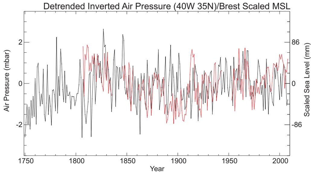
**Fig. 1.** Annual mean air pressure at  $40^{\circ}$  W,  $35^{\circ}$  N from the dataset of Küttel et al. (2009) shown in black, and annual mean MSL measured at Brest shown in red (the former measured Dec–Nov, the latter for calendar years). The air pressures have been multiplied by  $-1$  so as to correspond to sea level change. Both records have been detrended using a baseline period of 1807 onwards.
