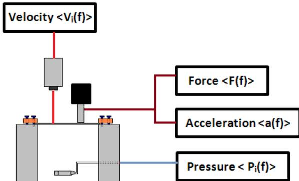
Figure 8. Experimental setup of the plate-cavity coupled structure. Subsystem frequency responses (plate velocity and cavity pressure) are simultaneously measured as the plate is excited. Force and acceleration at the drive point are also measured with an impedance head.
