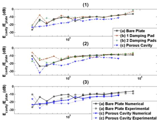
Figure 12. Subsystem energy ratio ( $E_{cavity}/E_{plate}$ ) in 1/3 octave bands for case (a), (b) and (c). (1) SmEdA predictions. (2) Experimental results. (3) Comparisons between SmEdA prediction and experimental results for case (a) and (c).
