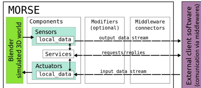
Fig. 1: Overview of the data flow in MORSE, between the simulated world in Blender and the external robotics software
