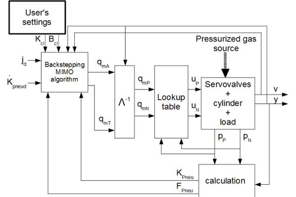
Fig. 2. Complete principle of the control strategy
