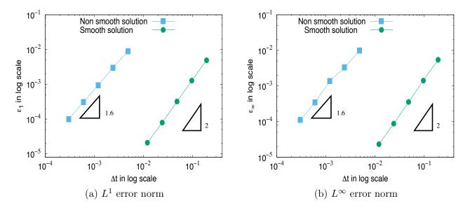
FIGURE 7. Test 4 - Hele-Shaw flow : (a)  $L^1$  error norm and (b)  $L^{\infty}$  error norm for the SSP-LDIRK2(3,3,2) L-stable scheme (24).
