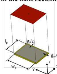
Figure 1. Phase reflection simulation of the patch unit-cell.
