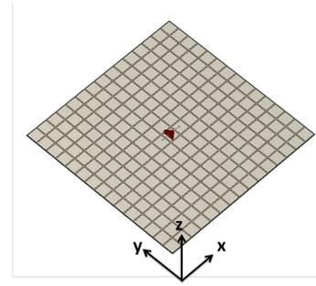
Figure 3. Dipole over a  $15 \times 15$  patches based HIS.
