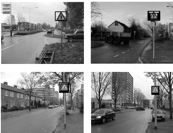
Fig. 14 Detection Results: warning and yield traffic signs
