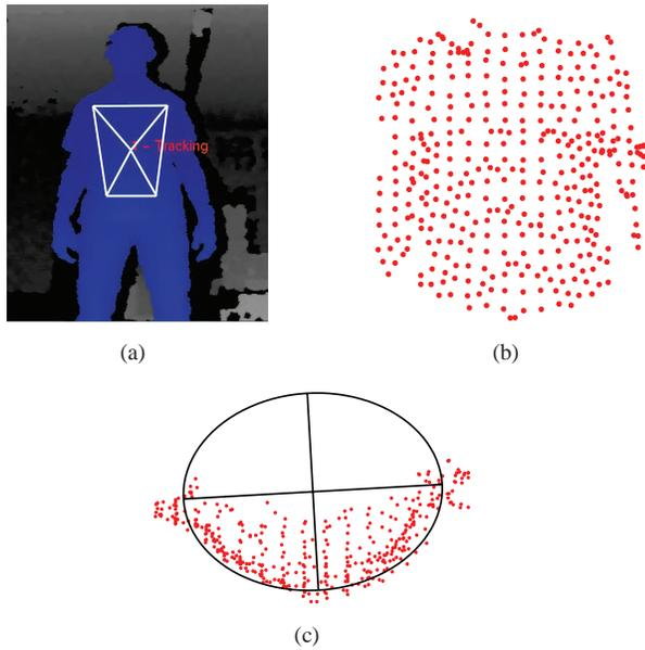
Fig. 5. *Human-body tracking on real data.* (a) NITE’s skeleton tracker is used to track the subject (the skeleton of the torso is shown in white). (b) The points which are not close enough to the torso are discarded, while the remaining points are down-sampled and expressed in the robot’s reference frame. (c) The points are finally projected onto the robot  $xy$ -plane and the position and orientation of the human body is determined via ellipse fitting.
