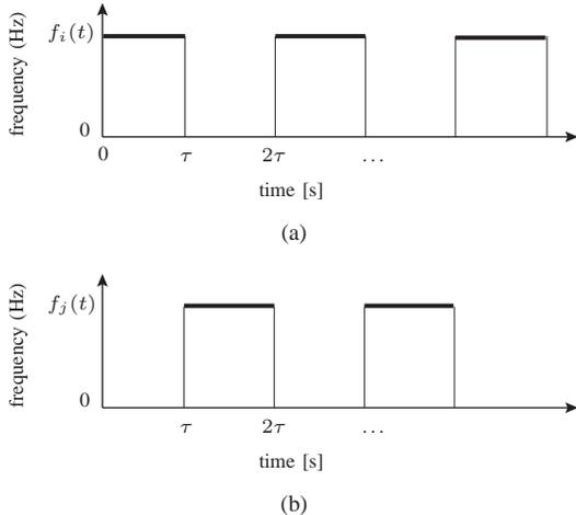
Fig. 4. *Temporization of the stimuli.* (a) In order to avoid the aftereffect problem, a periodic vibrational pattern with period  $2\tau$  is provided to the user. To keep signal recognition as simple as possible in the case of a combination of stimuli  $f_i(t)$ ,  $f_j(t)$  ( $i \in \{L, R\}$ ,  $j = C$ ), we alternate the patterns in (a) and (b).
