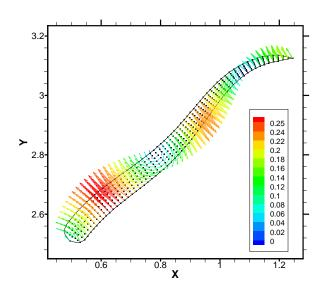
Figure 3: Lagrangian structured grid covering the fish after deformation and the corresponding velocity vectors of each point, colored by absolute velocity  $\sqrt{u^2 + v^2}$ .
