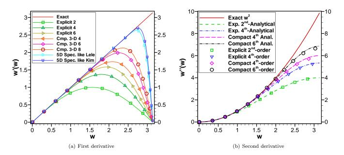
Figure 1: Plots of the scaled modified wavenumber for the first and second derivative, w'(w) and w''(w) respectively, versus the scaled wavenumber  $w = k\Delta x$  for different central finite difference methods presented in Lele [10] and Kim [23].
