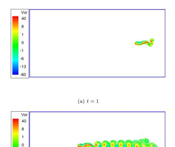
Figure 15: Snapshots of vorticity isolines obtained during a simulation where  $(x, y) \in [0, 10l_{\text{fish}}] \times [0, 5l_{\text{fish}}]$  by imposing a penalization parameter inside the body equal to  $\eta = 10^{-3}$  with resolution of 2048 × 1024, the Reynolds number is approximately  $Re \approx 3800$ .
