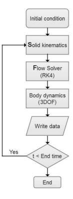
Figure 5: Flowchart of the fluid/solid interaction (FSI) algorithm.
