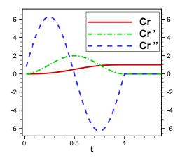
Figure 13: Smooth step function  $Cr(t) = t' - \sin(2\pi t')/(2\pi)$ ,  $t \in [t_i, t_f]$  with  $t' = (t - t_i)/(t_f - t_i)$ ,  $t_i = 0$ ,  $t_f = 1$  for gradually starting the motion proposed by Boyer et al. [21]. At t = 1 the left-and right-hand limits are equal for the function Cr and its first Cr' and second Cr'' derivatives.
