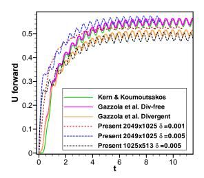
Figure 14: Forward velocity U of a 2D anguilliform swimmer's ( $\lambda = f = 1$ ). Solid lines indicate the reference simulations performed by Kern and Koumoutsakos (green) [22] and Gazzola et al. (pink and brown) [33]. Dashed lines represent the results with the proposed algorithm.
