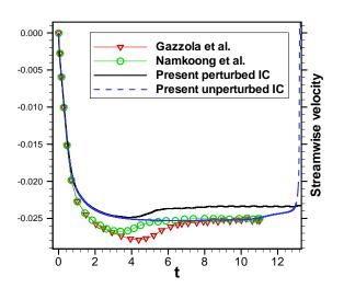
Figure 10: Comparison of the streamwise velocity of a falling cylinder via different methods/parameters. Symbols indicate the reference simulations performed by Gazzola et al. [33] (gradients) and Namkoong et al. [24] (circles). Solid and dashed lines represent the results with the proposed algorithm performed by a perturbed and unperturbed initial conditions (IC), respectively.
