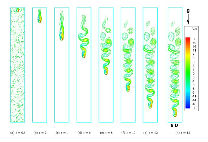
Figure 9: Vorticity isolines (dashed lines are used for negative values) of a falling cylinder in a slightly perturbed fluid,  $g = -9.81 \text{ m/s}^2$ ,  $\rho_b/\rho_f = 1.01$ , D = 0.005 m,  $(x, y) \in [0, 0.04 \text{ m}] \times [0, 0.32 \text{ m}] = [0, 8 \text{ D}] \times [0, 64 \text{ D}]$ ,  $\nu = 8 \times 10^{-7} \text{ m}^2/\text{s}$  and  $Re \approx 144$ .
