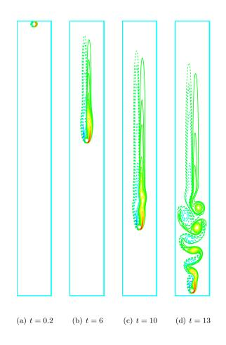
Figure 8: Vorticity isolines (dashed lines are used for negative values) of a falling cylinder in quiescent fluid,  $g = -9.81 \text{ m/s}^2$ ,  $\rho_b/\rho_f = 1.01$ , D = 0.005 m,  $(x, y) \in [0, 0.04 \text{ m}] \times [0, 0.32 \text{ m}] = [0, 8 \text{ D}] \times [0, 64 \text{ D}]$  and  $\nu = 8 \times 10^{-7} \text{ m}^2/\text{s}$  and  $Re \approx 156$ .
