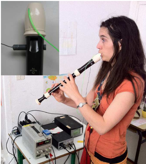
Figure 4: Experimental setup with the adapted recorder, allowing to measure both the pressure in the mouth of the flutist and the acoustic pressure under the labium.
