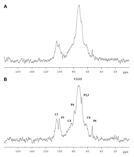
Fig. 3. Carbon CPMAS spectra of re-hydrated alcohol-insoluble residue (AIR) from apple tissues non-impregnated (B) and vacuum-impregnated with PME and calcium, maintained at 40  $^{\circ}$ C for 20 min and then pasteurized (A). C1–C6 correspond to signals attributed to cellulose, P1–P6 to signals attributed to pectins (P6 being the carbon of the methyl ester).
