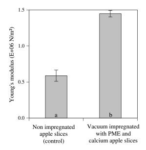
Fig. 2. Young's modulus obtained by a compression test of apple slices (2 cm diameter and 0.8 cm height) after vacuum-impregnation with PME (90 nkat  $g^{-1}$ ) and calcium (0.5% (w/w) CaCl<sub>2</sub>, 2H<sub>2</sub>O solution) (a) or no treatment (control) (b). The test was performed after the slices were maintained at 40 °C for 20 min and then pasteurized. Errors bars correspond to standard deviation (n = 20).
