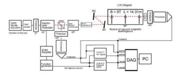
Figure 1: Set-up for the measurement of the Gas Magnetic Birefringence.
