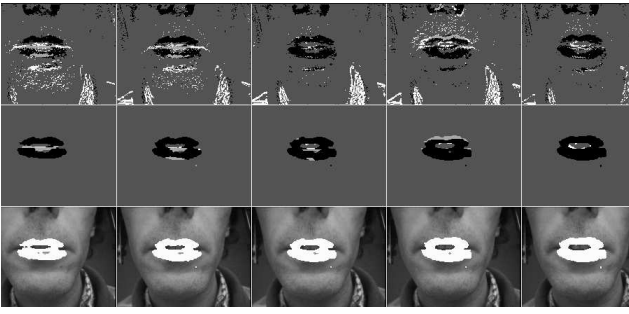
Figure 5: From top to bottom: initial labels; label fields after relaxation, The 4 labels are shown in grey levels (from white to black: b_1 , a_1 , b_0 , a_0 ); red hue relevant label images ( a_0 and a_1 ) superposed with luminance.
