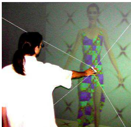
Figure 8: Using the SPIDAR for fashion design : human-scale haptic interaction with a virtual mannequin.
