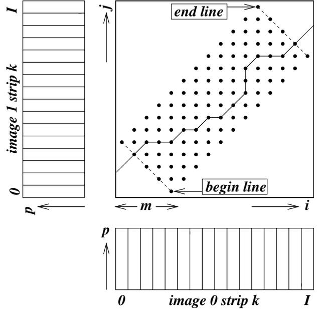
Figure 5: Dynamic Programming. Image strips and the matching path in the disparity matrix.
