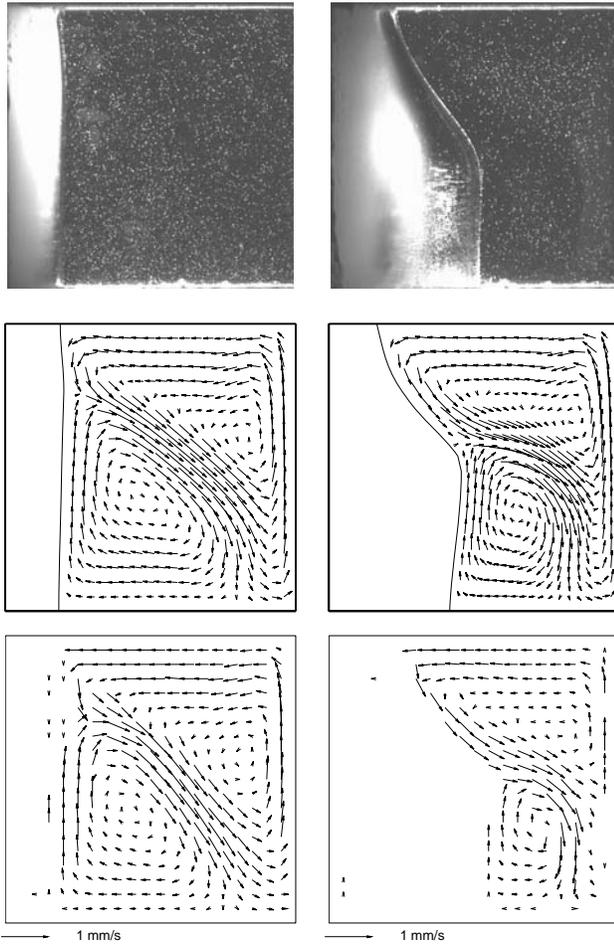
Figure 10: Freezing in the differentially heated cavity. Velocity fields at two time steps: 660s (left) and 100min (right) after initiating the flow;  $496 \times 496$  pixel particle images (top row), numerical calculations (middle row), DPIV evaluated vectors (bottom row), for pairs of images taken at 1.5s intervals
