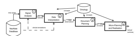
Figure 4: Architecture of BT-45.
