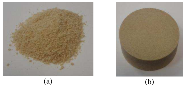
Fig. 3. Picture of the powdered foam (a) and pressed foam (b)
