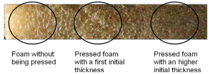
Fig. 7. Stepped sample after being pressed at 5mm.
