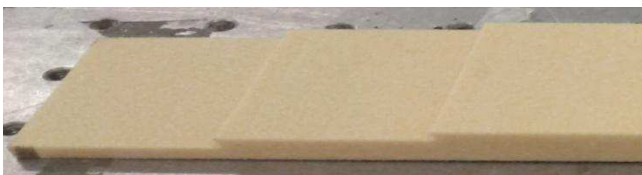
Fig. 6. Stepped sample before being pressed (5, 10, 15mm).
