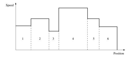
Figure 1: Decomposition of the track according to the maximal speeds
