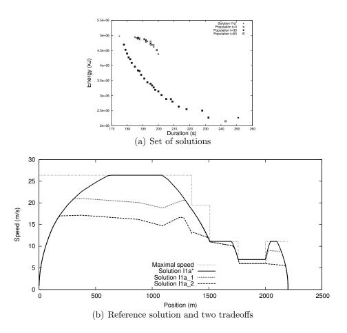
Figure 12: Results obtained on instance 1a: (a) Fronts of solutions at times  $t=\{0, 30, 60\}$  for outward journey; (b) Examples of speed profiles for outward journey.
