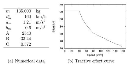
Figure 11: Technical parameters of train AGC
