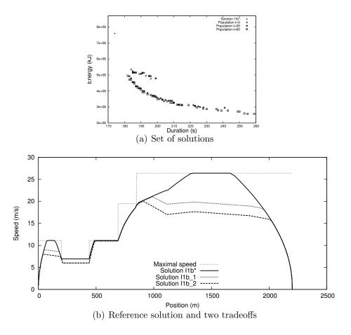
Figure 13: Results obtained on instance 1b: (a) Fronts of solutions at times  $t=\{0, 30, 60\}$  for inward journey; (b) Examples of speed profiles for inward journey.
