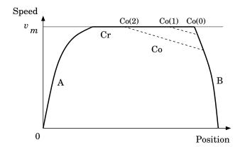
Figure 2: Usual speed profile over one section in four steps (assuming no slope): acceleration (A), cruising (Cr), coasting (Co) and Braking (B).
