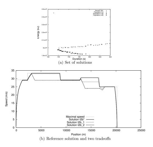
Figure 15: Results obtained on instance 2b: (a) Fronts of solutions at times  $t=\{0, 30, 60\}$  for inward journey; (b) Examples of speed profiles for inward journey.
