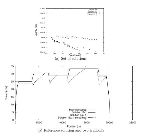
Figure 14: Results obtained on instance 2b: (a) Fronts of solutions at times  $t=\{0, 30, 60\}$  for inward journey; (b) Examples of speed profiles for inward journey.
