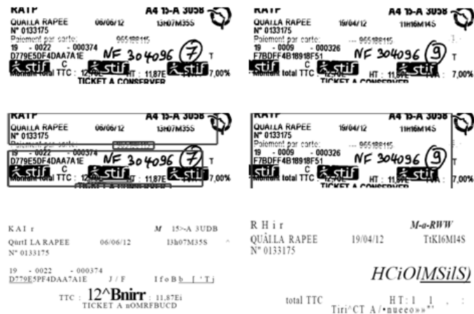
Fig. 2. Complexity of text and layout extraction: two original images from "RATP" class (row 1), the extracted structures (row 2) and the OCR results (row 3). The layout and the OCR are carried out by FineReader 10. For these two very similar documents, the layout and text extracted are very different.
