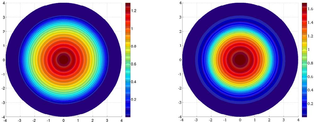
Figure 1: Numerical simulations for component  $u$  in (1). (1) Left: Plot of the computed  $u$  at time  $T = 1$  for  $\alpha = 0.25$  and  $\theta = 0.1$ . (2) Right: Plot of the computed  $u$  at time  $T = 3$  for  $\alpha = 0.25$  and  $\theta = 0.5$ . In both cases, we observe the propagation of a stable spherical wave which invades the computational domain.
