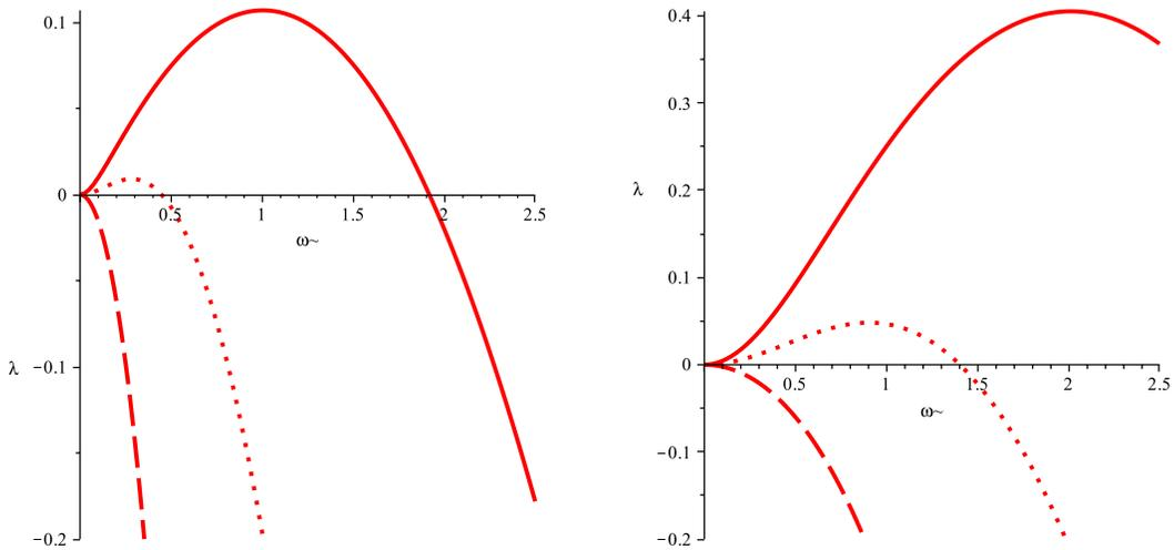
Figure 6: (Left) Plot of the dispersion curve  $\lambda(\omega)$  for  $\theta = 0.4$  and  $\alpha = 0.1$  (continuous line),  $\alpha = 0.4$  (dotted line) and  $\alpha = 1.3$  (dashed line). (Right) Plot of the dispersion curve for  $\theta = 0.1$  and  $\alpha = 0.1$  (continuous line)  $\alpha = 0.2$  (dotted line)  $\alpha = 0.4$  (dashed line).
