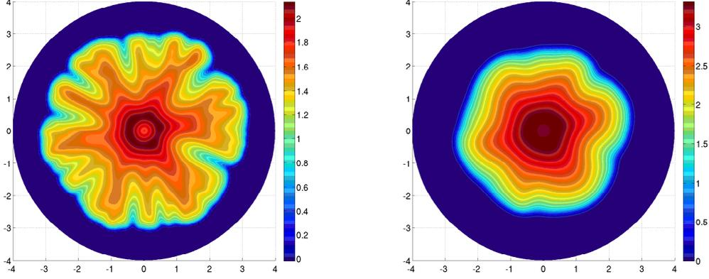
Figure 2: Numerical simulations for species  $u$  in (1). (1) Left: Plot of the computed  $u$  at time  $T = 2$  for  $\alpha = 0.01$  and  $\theta = 0.1$ . (2) Right: Plot of the computed  $u$  at time  $T = 6$  for  $\alpha = 0.25$  and  $\theta = 0.5$ . When  $\alpha$  is small, numerical instabilities appear which create a complex fingered pattern.
