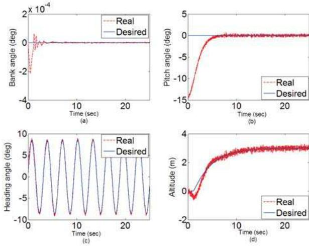
Fig. 11. Desired trajectories tracking for uncertainties of 20% on  $m$  and 10% on  $(I_x, I_y, I_z)$
