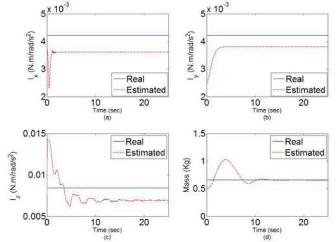
Fig. 14. Inertia matrix and mass estimation for uncertainties of 35% on  $m$  and 15% on  $(I_x, I_y, I_z)$
