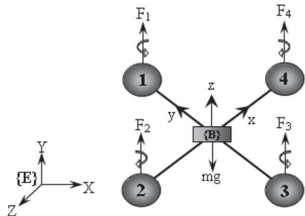
Fig. 1. Quadrotor Configuration
