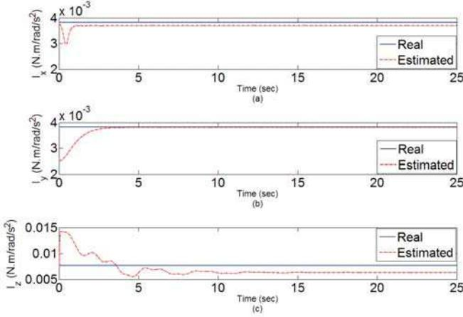
Fig. 4. Simulation results of inertial moments estimation
