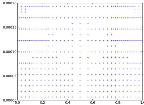
FIGURE 5. An example of an inhomogeneous mesh of the space of parameters (with 500 points). The two parameters are  $w = D/R$  and  $x_0$ . We can see that the finer zones have a smaller size than the size the homogeneous mesh of Figure 4 (which contains 1089 points): the mesh is here more refined in zones where the model has strong variations and coarsened in zones where the variations are small.
