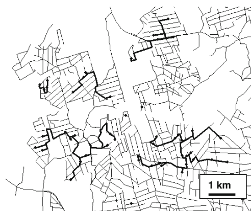
Fig. 5 The deletion of distances greater than 3,000 m from the minimum spanning tree results in clusters ( bold black lines ) of stand identifiers or harvest stands respectively. Three of them are individual clusters ( black points )
