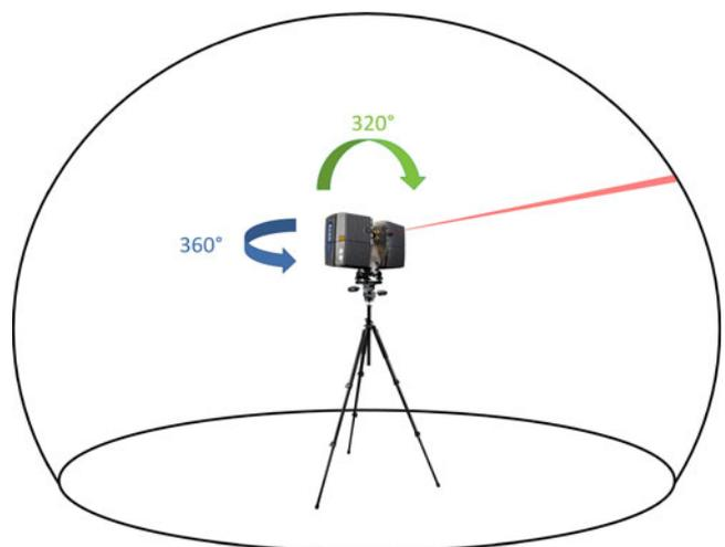
**Fig. 1** Operating principle of a terrestrial LiDAR (light detection and ranging) scanner (FARO Photon 120). A laser beam deflected by a rotating mirror scans a vertical plane, and the complete rotation of the device allows hemispherical scanning. This results in the digitisation and the representation of surrounding objects in a three-dimensional (3D) point cloud
