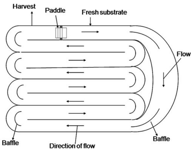
Fig. 2 Aerial view of a raceway pond
