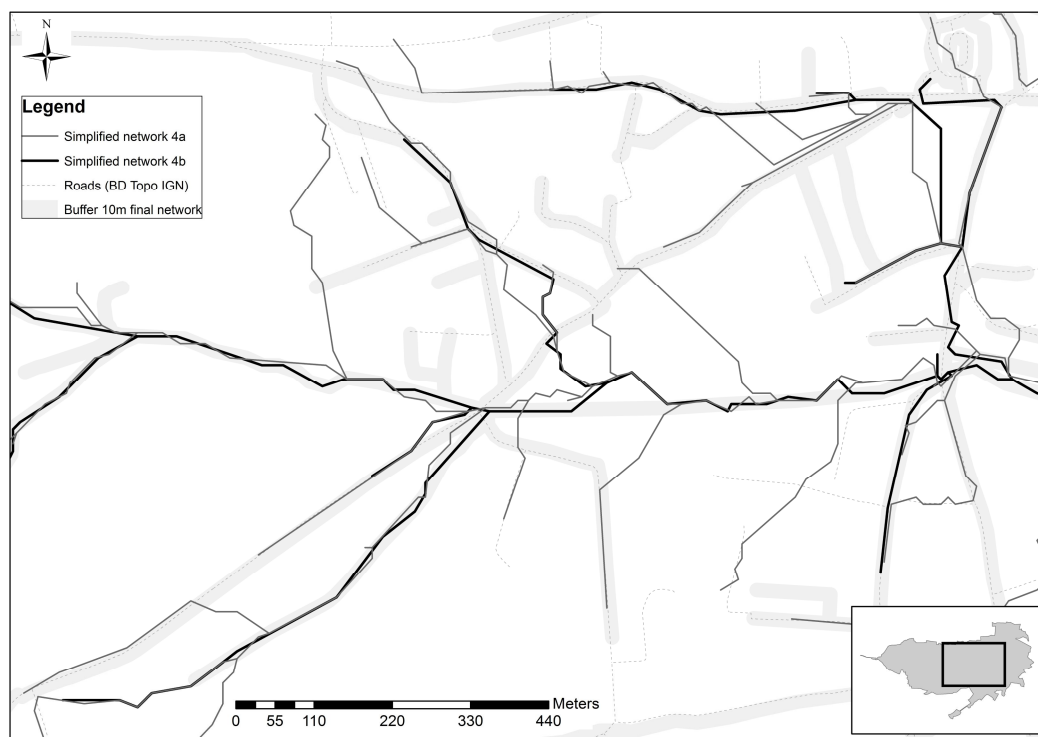
Figure 8: Visualization of the network agreement criterion, which represents the network length falling inside a buffer of 10 meters around the total network (i.e. combined sewer system, rainwater network and the natural stream). Drainage networks of Methods 4a (only based on the road network) and 4b (using road, combined sewer system and natural stream) are compared to this buffer and the road network. Method 4b reduces the network density and enhances thus the agreement with the real network (buffer), but detects less roadside ditches or pipes.
