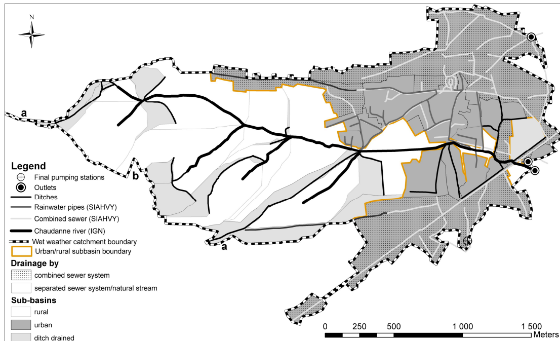
Figure 7: Final map of subcatchments. Urban subcatchments are in dark grey, rural subcatchments in white and subcatchments drained by ditches in light grey. The dotted subcatchments are only connected via stormwater overflow devices to the river. The subtraction of the dotted area from the wet catchment area results in the dry catchment area. Locations a and b indicate areas of special interest.
