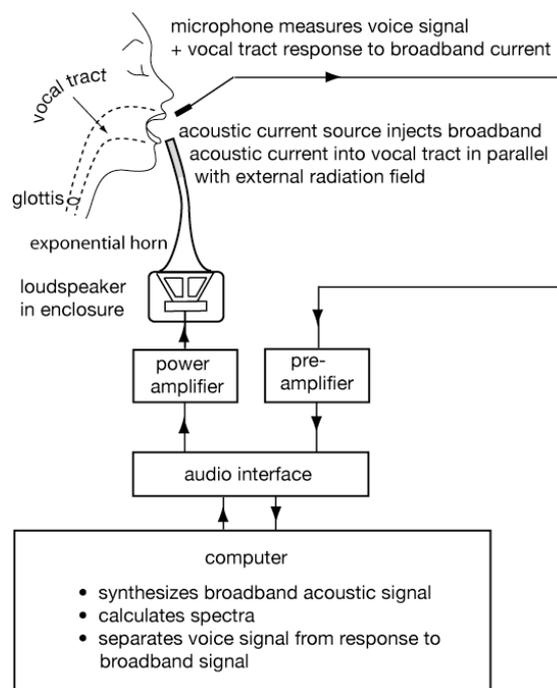
**Figure 1.** Schematic diagram (not to scale) showing the technique used for real-time measurement of vocal tract resonances. The microphone is normally mounted alongside, and parallel with, the end of the acoustic current source; in this diagram they have been separated for clarity.
