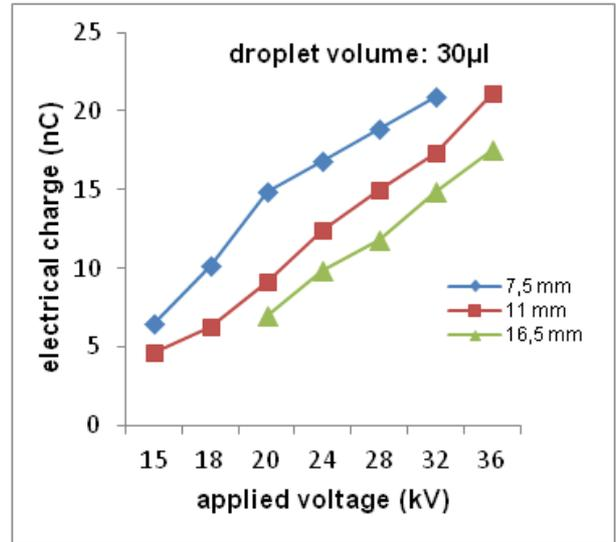
Figure 3: effect of applied voltage on the estimated electrical charge for various inter-electrode distances in rod to plane system.
