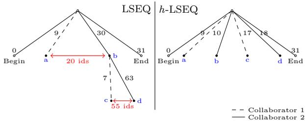
Figure 2: Representation of the underlying exponential tree model of LSEQ and  $h$ -LSEQ. Two collaborators insert two elements at the end of the document in order to get the sequence “abcd”. On the random side, the collaborators employ antagonist strategies. On the hash side, the collaborators use the same allocation strategy. Both sides draw the same random numbers.
