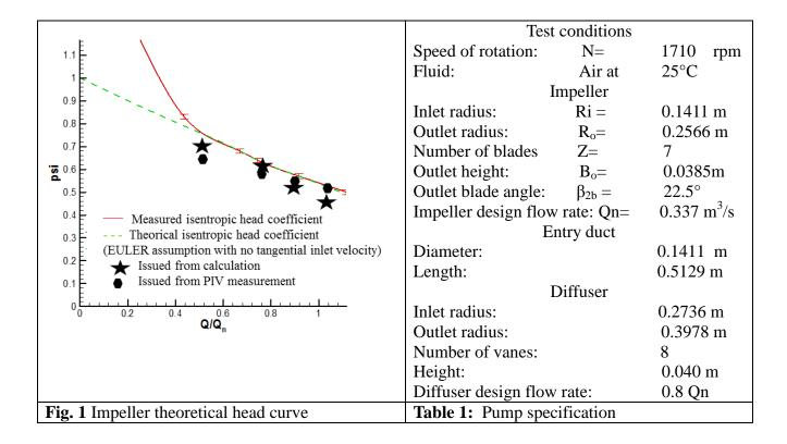
The main features of the components and specifications of the considered operating condition are summarized in Table 1. The particular mass flow rate of Q/Qn = 0.774 corresponds to an off design condition for the impeller and a near design condition for the vaned diffuser. The choice of a different design condition for impeller (Q/Qn close to 1.) and diffuser was intended to improve performance at low flow rates for the whole pump.
