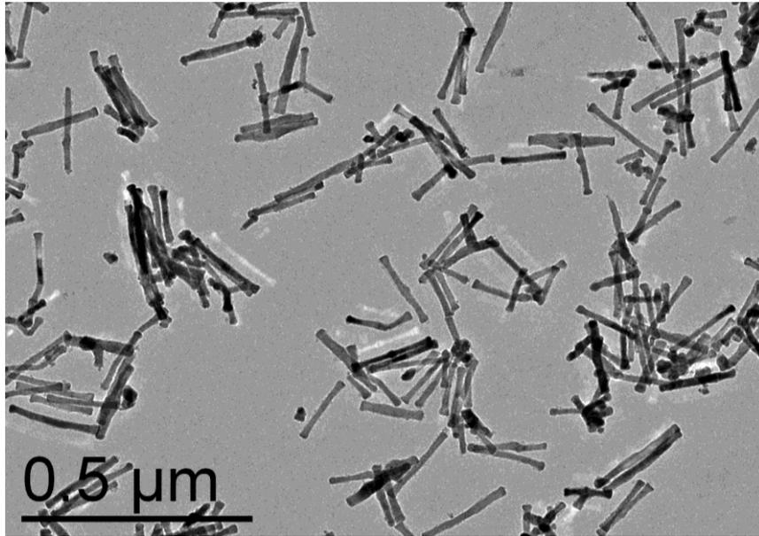
**Figure 9** TEM image of carbon coated Co nanorods annealed at 400 °C under N<sub>2</sub> (O<sub>2</sub> < 0.1 ppm) for 2h.
