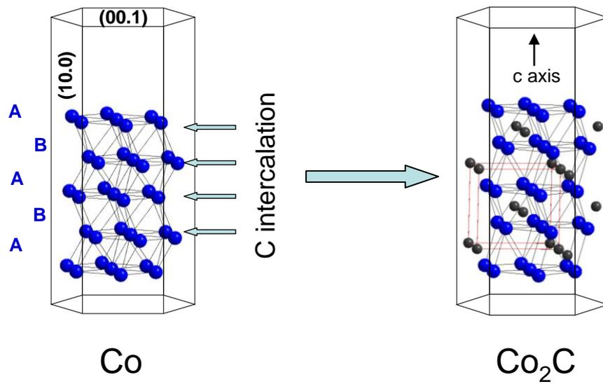
**Figure 11.** Scheme of formation of a  $\text{Co}_2\text{C}$  grain in a cobalt rod by intercalation of C atoms from the  $(10\bar{1}0)$  sides of the hcp Co.
