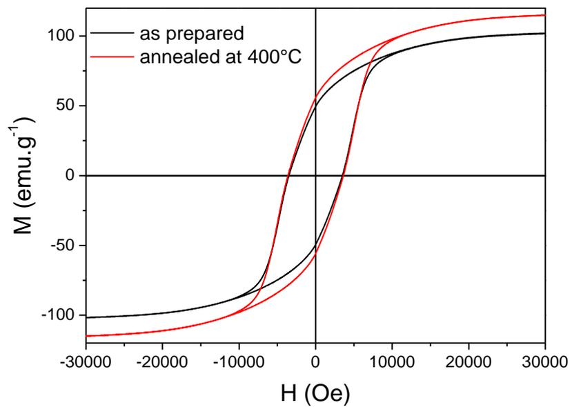
**Figure 10.** Room temperature magnetization curve of carbon coated Co nanorods (black) and of the same coated rods annealed at 400 °C under N<sub>2</sub> (O<sub>2</sub> < 0.1 ppm) for 2h (red).
