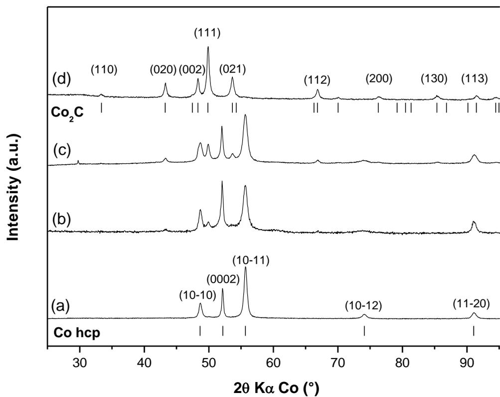
**Figure 4** XRD pattern of Co rods treated (a) in ODE for 3h and in a mixture of ODE/OA for (b) 30 min, (c) 3h and (d) 4h (only the  $Co_2C$  strongest lines are indexed).
