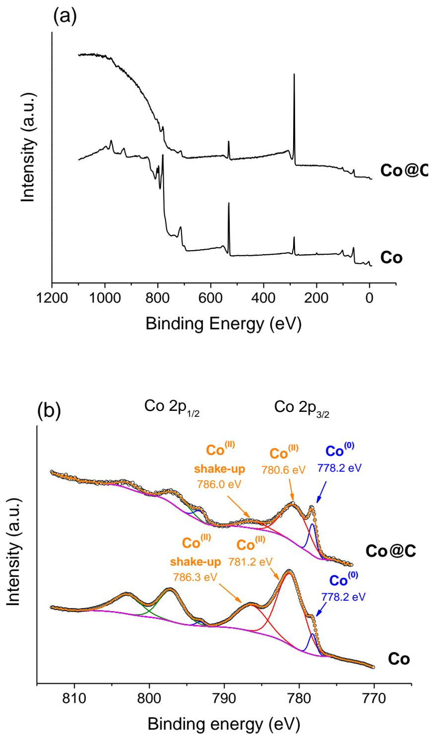
**Figure 3** X-ray photon electron spectra of cobalt rods and cobalt rods coated by a thin carbon shell by a treatment in ODE at 300°C for 3h: (a) survey scans ; (b) Peak fitting of Co 2p peak high resolution scans.
