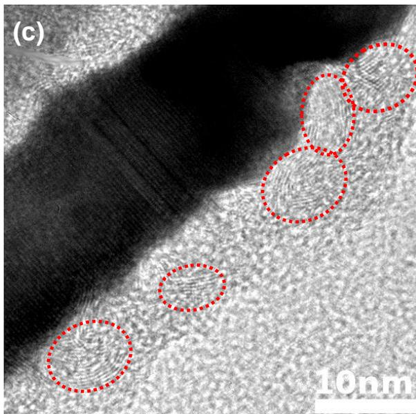
**Figure 2** (a) SEM, (b) TEM and (c) HRTEM images of cobalt rods coated with a thin carbon shell by a treatment in ODE at 300 °C for 3h (the circles indicate local onion structure with a distance in the range 3.4-3.5 Å).
