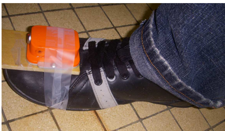
Fig. 10 Inertial Measurement Unit MTi attached to the foot of a subject during displacement
