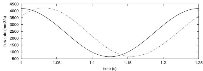
FIGURE 3. Time evolutions of the flow rate at sections  $\text{—}$  :  $x = x_{\text{inlet}}$  and  $\text{⋯}$  :  $x = x_{\text{outlet}}$  for the case R2. Note that the origin of time is 1 s since the fifth cycle is analysed (see text).
