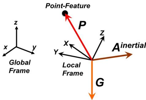
**Fig. 1** Global and local frame with the point-feature position ( $\mathbf{P}$ ), the platform acceleration ( $\mathbf{A}^{inertial}$ ) and the gravitational acceleration ( $\mathbf{G}$ ).
