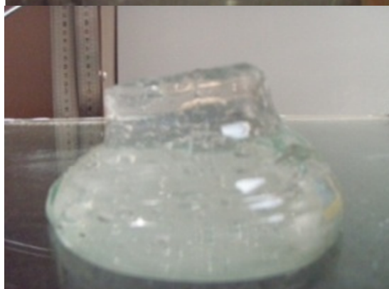
Figure 2. Images of Carbopol ® dispersions at the flow stoppage. Values of suspension yield stress: a) 21 Pa; b) 28 Pa; c) 62 Pa; d) 100 Pa.
